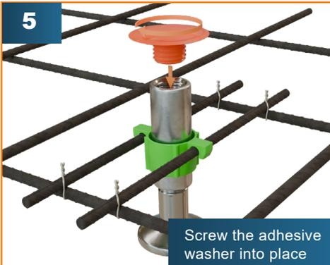
Screw the adhesive washer into place
